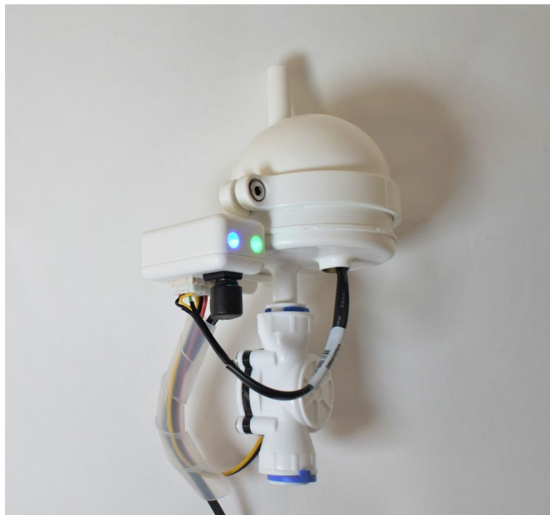
Figure 3-22: Flow Sensor Package with External Indicators
